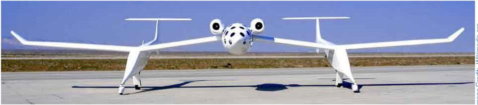
**White Knight I** Virgin Galactic intends that an enlarged version of this aircraft, White Knight II, will carry a SpaceShipTwo into the stratosphere for launch. Effectively it is the first stage of a two-stage space launcher .
